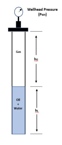
Wellhead Pressure = 350 psia Fluid Level = 844 ft Formation Depth = 1,678 ft Oil Gravity = 36 API Water Sp. Gr. = 1.03 Average Oil Cut = 42% Formation Temp = 83 °F Surface Temp = 70 °F Gas Sp. Gr. = 0.72 To obtain the bottom-hole pressure, one calculates the pressure due to the compressed gas column and the oil+water column and add them together. Each of these calculations is independent of each other and can be easily calculated.
